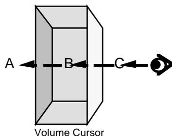
Figure 2: Using a "silk" covering over a rectangular volume cursor in order to obtain occlusion-based depth cues. An object at point A is seen through two layers of "silk", and so is perceived to be *behind* the volume cursor. An object at point B is seen through one layer, and so is perceived as *inside* the cursor's volume. An object at point C is not occluded by the silk at all, and so is seen to be *in front* of the volume.
